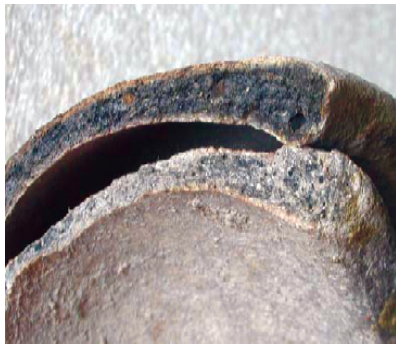
Figure 13: Edges of broken bowl fired at inconsistent temperatures.
