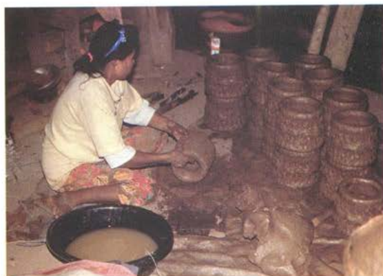
Figure 25. Potter Mrs. Saun shaping a hollowed-out cylinder to make a vessel preform. The bamboo stick used to pierce the center of the cylinder lies to the potter's left. These cylinders will be used in stacked pairs to make large vessels. Northeast Thailand, Khon Kaen, Nam Phong, Wang Thua, 1995.
