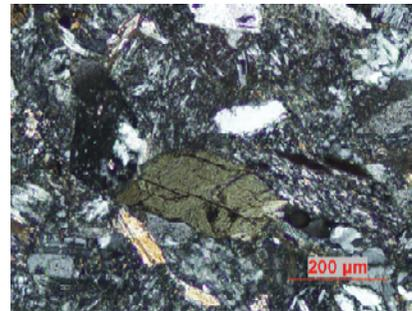
*Figure 6: micrograph 4 amphibole*
