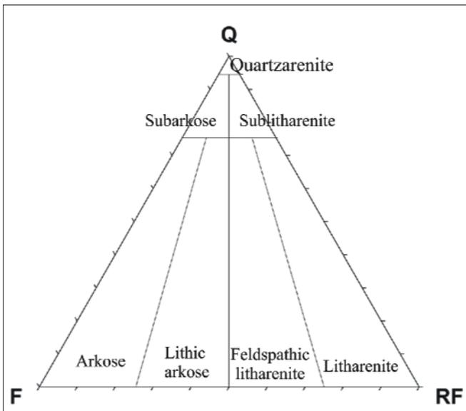
Figure 2: Classification scheme of sandstones after Folk 1974.
